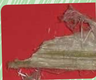
Chrysotile asbestos (white).
