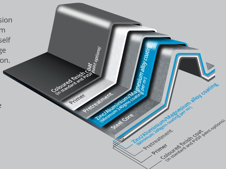
Suitable for moderate climatic environments, ZinaCore has a hot-dipped aluminium/zinc alloy coated steel substrate. It has a water-borne or polyester top coat baked on a polyester primer, giving an extremely durable paint system that resists UV damage and provides excellent gloss and colour retention.
